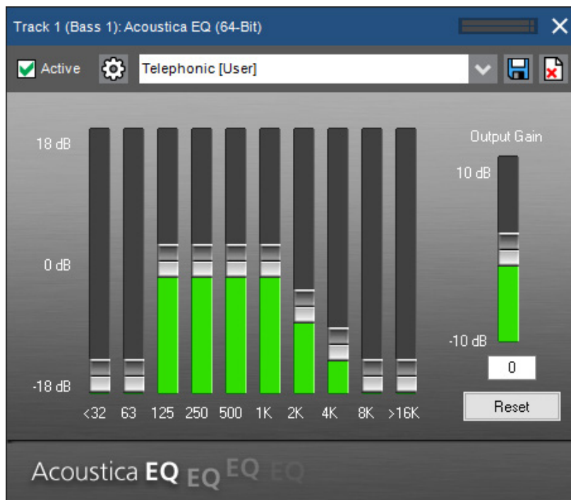
Acoustica's EQ. The sliders change the volume of the frequency bands.
