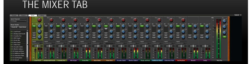
The Mixer Tab displays a virtual display of a standard mixing console. Used by many as part off the "final mixdown", you can control: volume levels; pan tracks left, right or center; mute or solo tracks.
