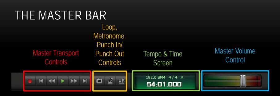
Master Transport Control – (from left to right) – record, rewind to beginning, rewind portion, play, fast forward portion, fast forward to end. Shortcuts – Spacebar=play/stop, R=record
